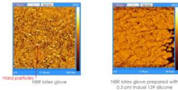
Figure 8. Surface Hardness Measured by AFM (The lighter the color, the harder the surface)
